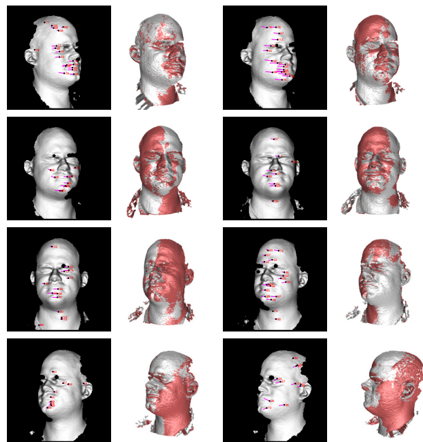
Figure 8. All pairwise coarse registrations in the Rick1 sequence. Wrong correspondence 26 on the lip in the last pair caused a slight registration bias that shows around the nose.
