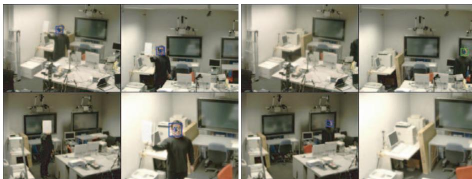
(a) Robust tracking when the one camera cannot observe the subject due to occlusion
