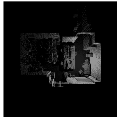
Fig. 2. Three-dimensional shape of an environment measured by using a range finder.
