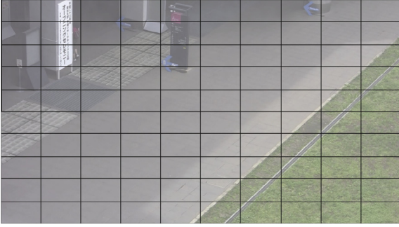
Fig. 5. An example of dividing a scene into 10 \times 10 unit regions ( K = 100 ). These regions serves as the smallest unit to construct each region.
