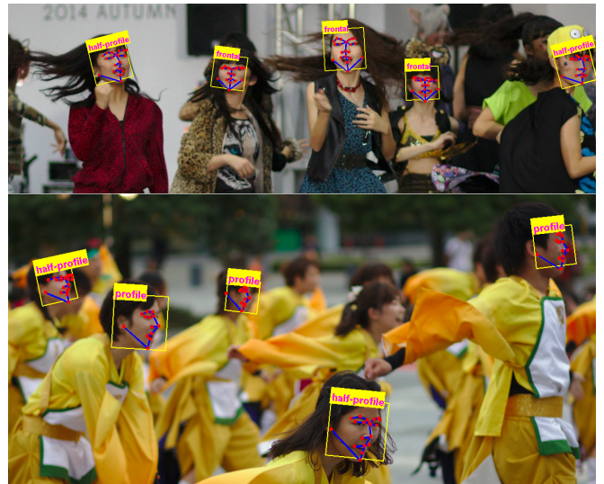
Fig. 1. The exemplary output of our proposed detector. The yellow boxes are detections provided by the face detector. The red dots represents the landmark, the blue lines shows the organization of the underlying graph for a detected view (i.e. the discretized yaw angle), which is written on the top of the detected face bounding box in magenta.
