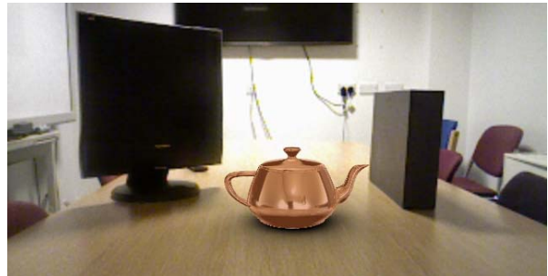
Figure 1: Image augmented with virtual reflective teapot, rendered using the proposed system. Note the reflections of the nearby real objects. No physical light probe was placed near the teapot.
